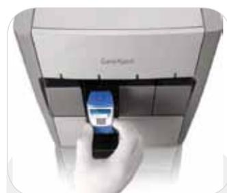
Sputum is placed into a cartridge and then into the Gene Xpert.
